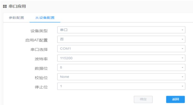
The screenshot shows the 'Serial Application' configuration page. It has two tabs: 'Parameter Configuration' and 'Configuration from Device'. The 'Configuration from Device' tab is active. The configuration items are as follows:
