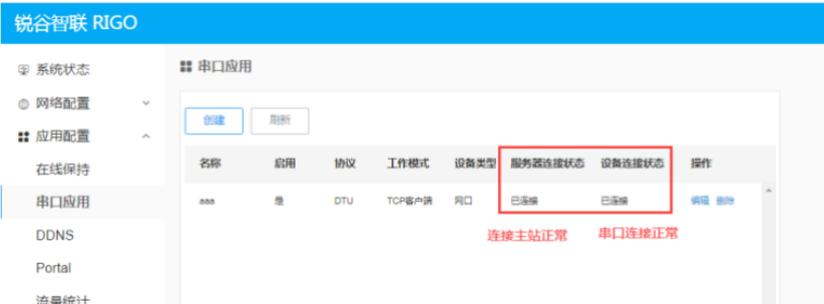
The screenshot shows the 'Serial Application' management interface. On the left is a navigation menu with '应用配置' (Application Configuration) selected. The main area shows a table of serial applications. A red box highlights the '服务器连接状态' (Server Connection Status) and '设备连接状态' (Device Connection Status) columns. Below the table, red text indicates '连接主站正常' (Main Station Connection Normal) and '串口连接正常' (Serial Port Connection Normal).
